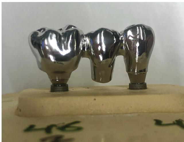
**Figure 1.** Experimental model: 2 implants parallel to each other, 2-mm abutment placed in first molar position, and 3-mm abutment placed in first premolar position. CAD-CAM superstructure tightened to both abutments. CAD-CAM, computer-aided design and computer-aided manufacturing.
