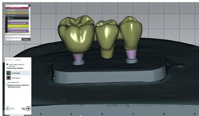
**Figure 3.** Virtual abutments placed with computer-aided design software into virtual implant replicas. Designed digital superstructure then placed on virtual abutments
